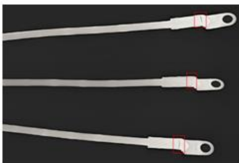
Fig. 4 100kV at 3 × 70mm cable ends
