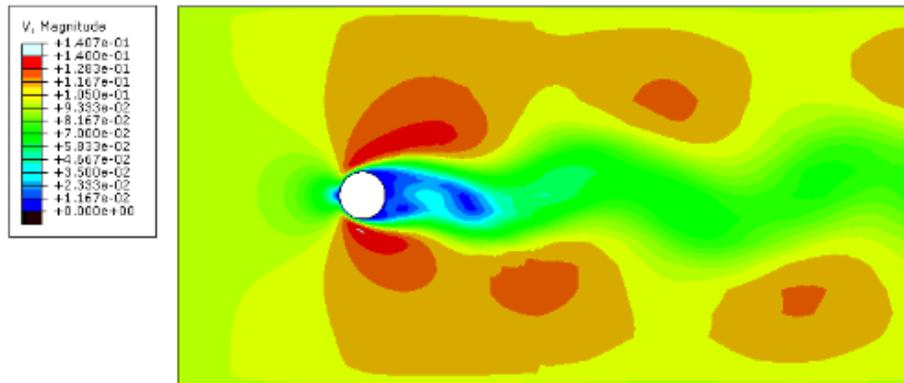
Figure. 3-3 single cylinder speed cloud - vortex shedding ( $t = 2s$ )
