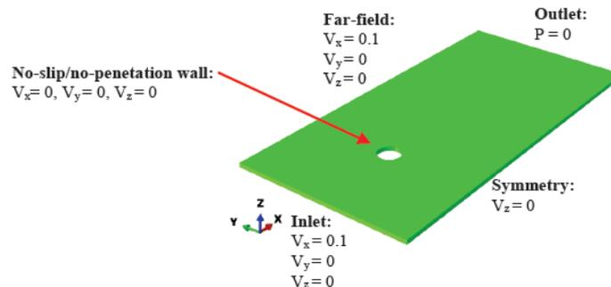
Figure.2-3 the boundary conditions of the Single cylinder flow
