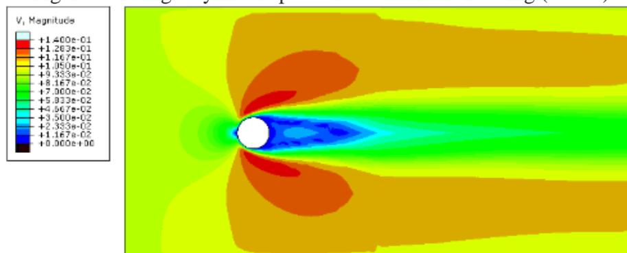
Figure. 3-2 single cylinder speed cloud - vortex shedding (t = 1s)
