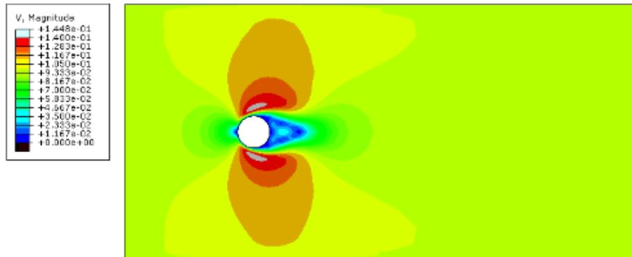
Figure. 3-1 single cylinder speed cloud - vortex shedding (t = 0 s)
