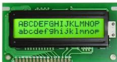
Fig. 1 Typical character liquid crystal module real object diagram
