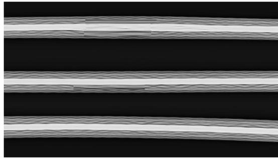
Fig.2 Steel core off shares simulated defect detection
