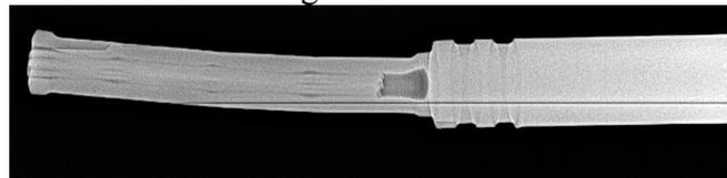
Fig.5 Crimp depth insufficient simulated defect detection
