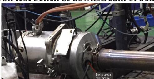
Figure 4 Layout of NOx test bench at downstream of barrel-type post-treatment
