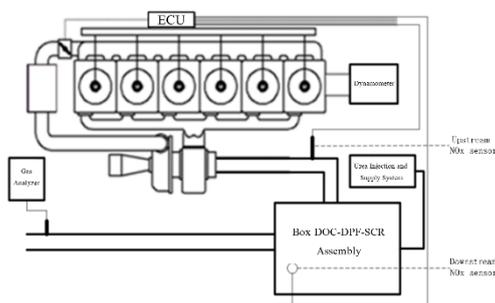
Figure 1 Layout diagram of NO<sub>x</sub> test downstream of box-type post-treatment
