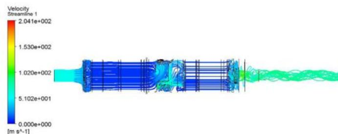
Figure 14 Air flow path of rear chamber booster
