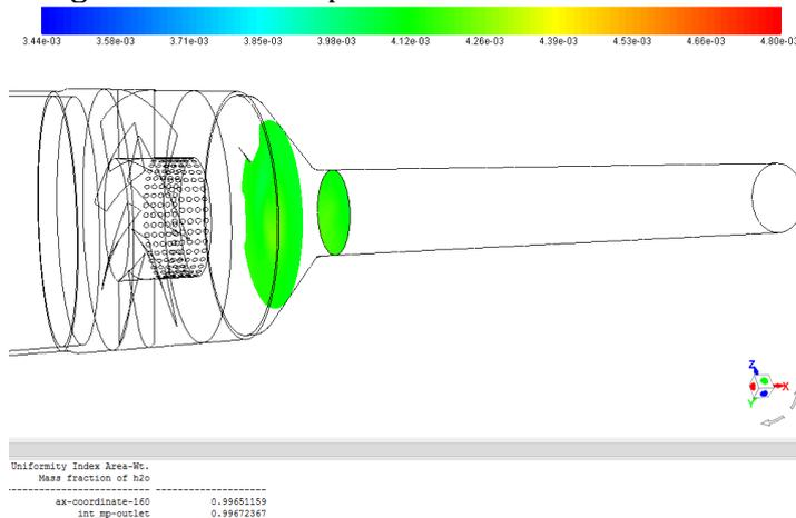
Figure 15 Ammonia uniformity of rear chamber booster
