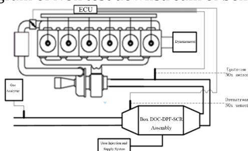
Figure 2 Layout diagram of nitrogen and oxygen test downstream of barrel-type post-treatment
