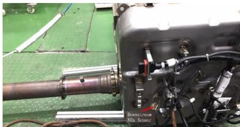
Figure 3 Layout of NOx test bench at downstream of box-type post-treatment
