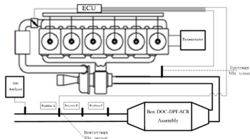
Figure 11 Layout diagram of nitrogen and oxygen test bench at downstream of barrel post-treatment
