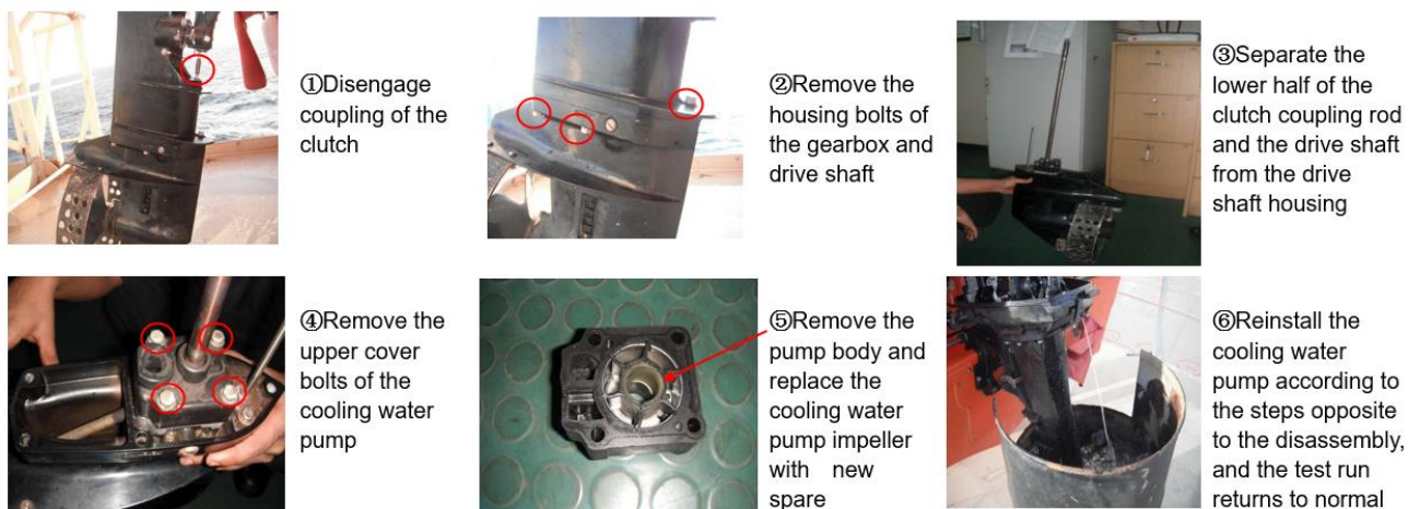
Fig.2 Cooling water pump impeller renewed
