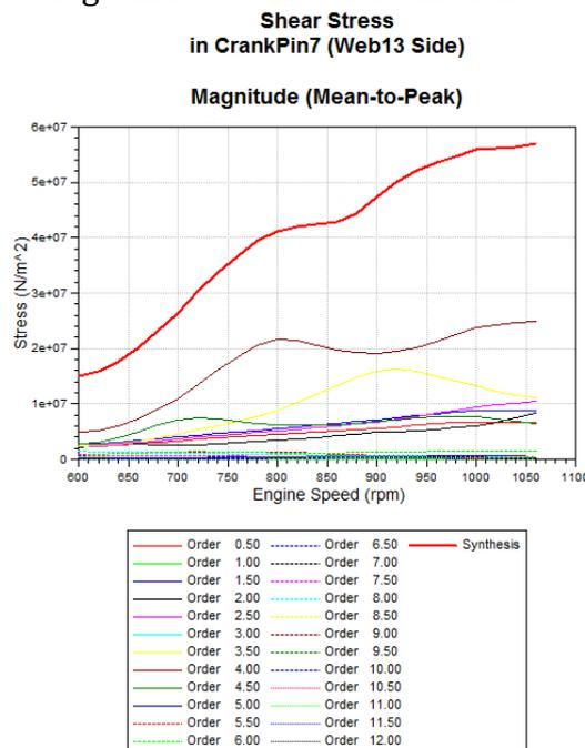
Fig.8 Torsional vibration stress results
