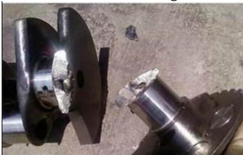
Fig.1 Crankshaft torsional fracture
