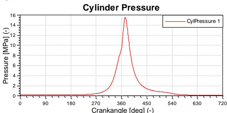
Fig.5 Cylinder pressure test data
