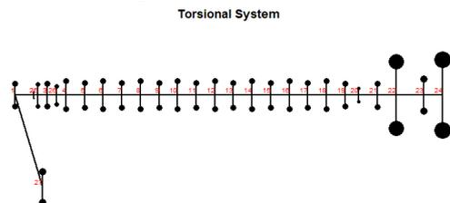
Fig.4 Shaft system equivalent model
