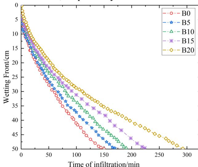
Fig.3 Dynamic changes of wetting fronts under different biochar application rates
