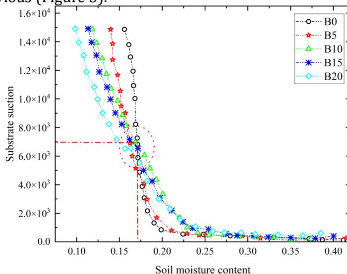
Fig.5 Soil moisture characteristic curves of different biochar treatments
