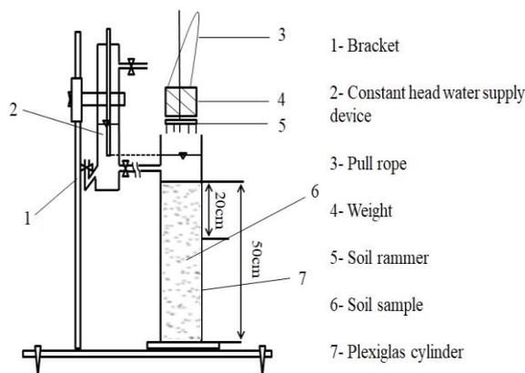
Fig.1 Schematic diagram of vertical soil column infiltration test setup
