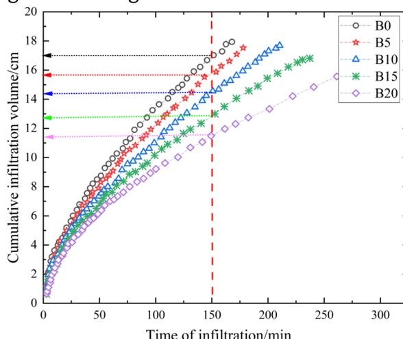
Fig.4 Effect of biochar application rate on cumulative infiltration
