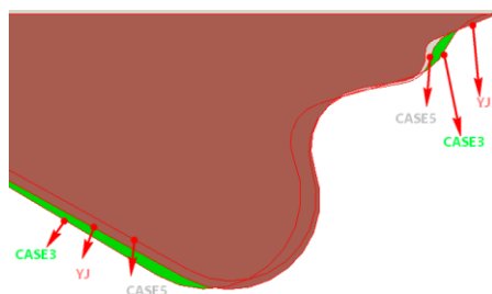
Fig. 12. Comparison of combustion chamber shapes of CASE 3, CASE 5 and the original engine
