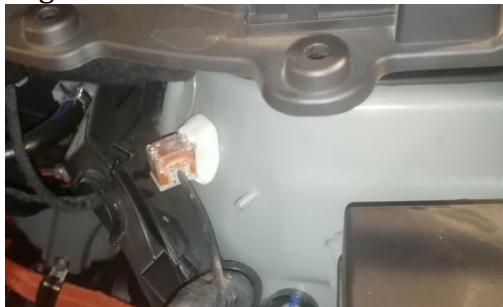
Fig. 6 Position of accelerator on topmount
