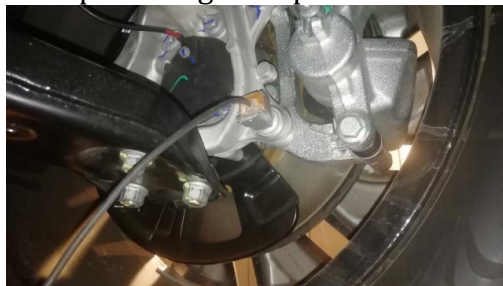
Fig. 5 Position of accelerator on axle
