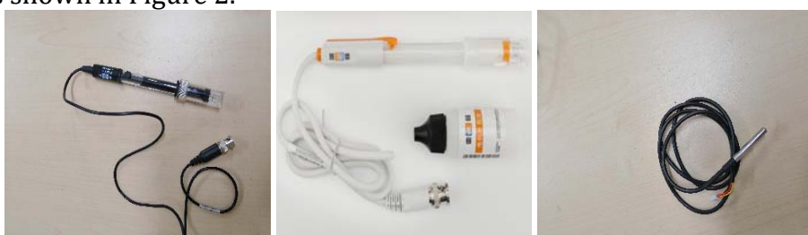
(a)TDS sensor (b)PH sensor (c)temperature sensor
