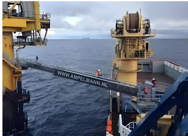
Fig. 4 Active Wave Compensation System for Offshore Ladders
