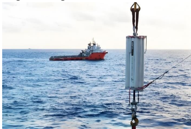
Fig. 3 Passive Wave Compensation System for Offshore Lifting Operations
