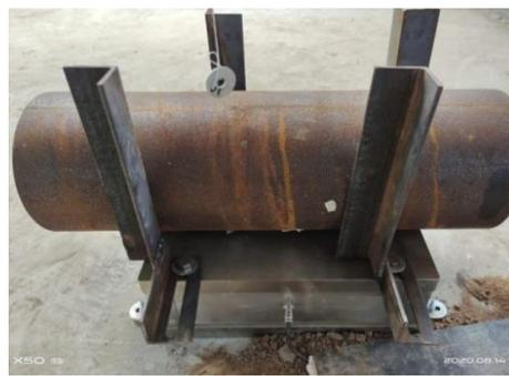
(f) Assembly drawing of oil and gas pipeline and force measuring platform
