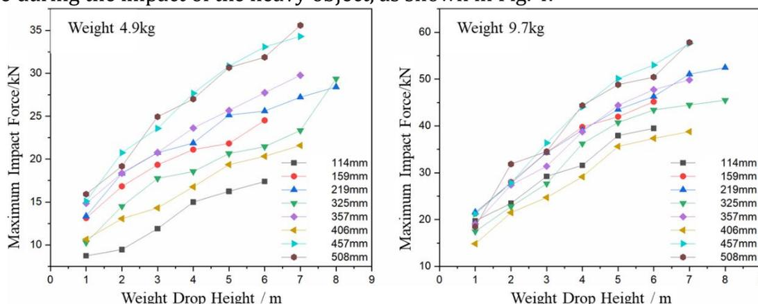
Fig. 4 Force Curve of Oil and Gas Pipeline during Impact by Heavy Object
