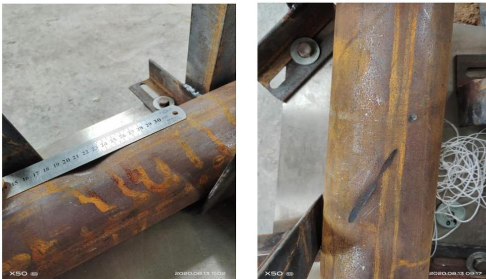
Fig. 3 Damage and Deformation of Oil and Gas Pipeline after Impact by Collapsing Heavy Objects
