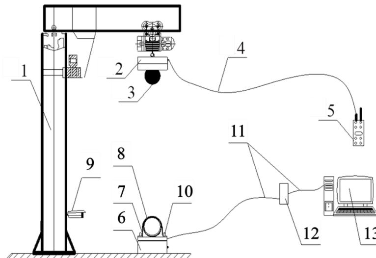
1- Cantilever Crane; 2- Automatic Unhooking Device; 3- Iron Ball; 4- Remote Control Wiring; 5- Remote Control; 6- Force Measurement Platform; 7- Fixing Device; 8- Steel Pipe; 9- High-Speed Camera; 10- Fixing Bolt; 11- Data Cable; 12- Data Acquisition Card; 13- Computer
