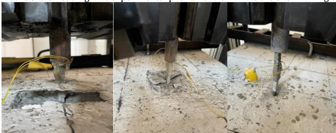
Fig. 6 R1 ~ 3 Failure Phenomenon
