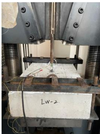
Fig.4 Test Loading Device
