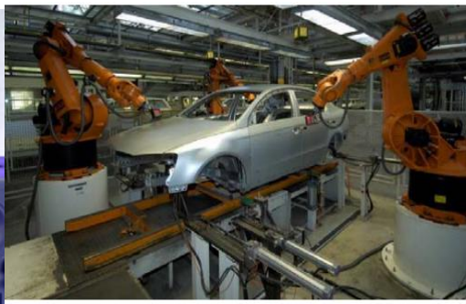
Fig. 5 Welding site of car body
