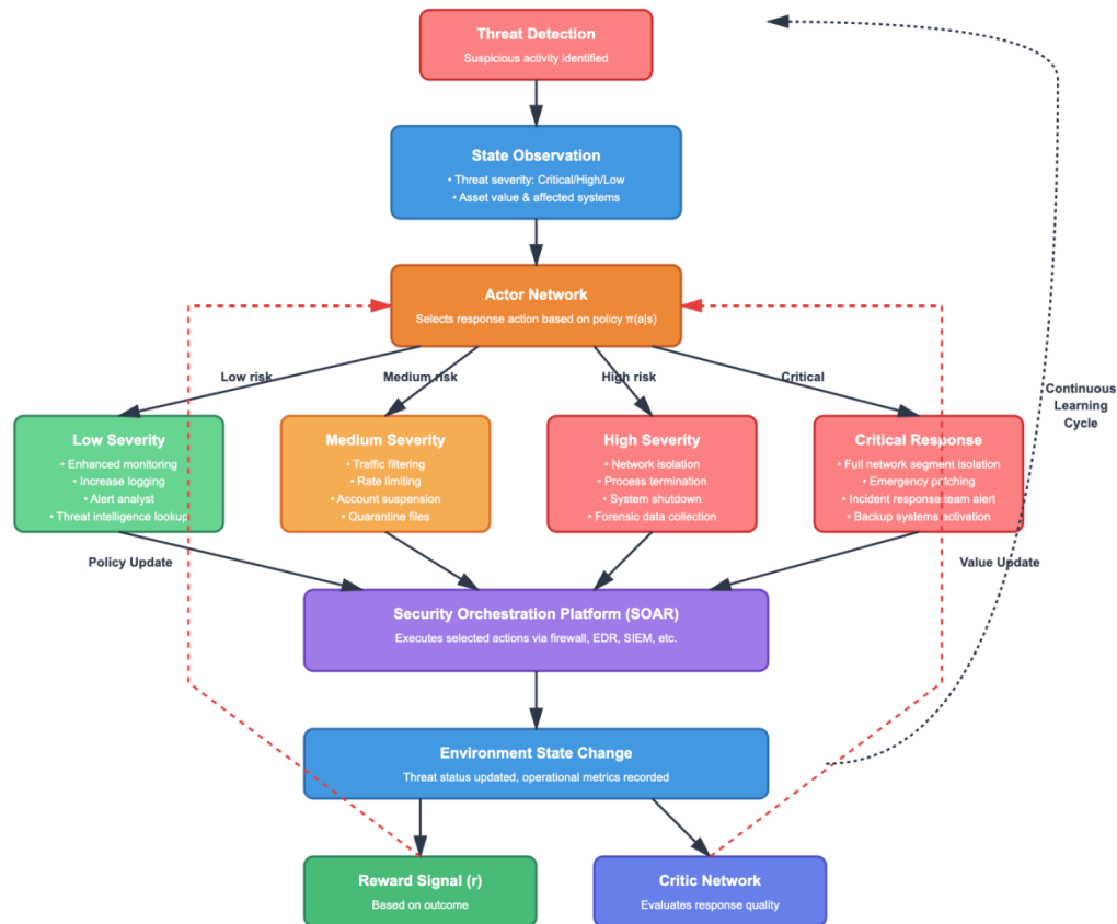
Figure 2. Flowchart depicting the automated incident response process using actor-critic reinforcement learning. When a threat is detected, the system generates a state observation including threat severity, asset criticality, and system status. The actor network selects appropriate response actions based on learned policy \pi(a|s) , ranging from low-severity monitoring to critical system isolation. Actions are categorized by severity: low-severity responses include enhanced monitoring and logging; medium-severity responses involve traffic filtering and account suspension; high-severity responses include network isolation and process termination; critical responses trigger full segment isolation and incident response team activation. Selected actions are executed through security orchestration platforms (SOAR) that interface with firewalls, endpoint detection and response (EDR) systems, and security information and event management (SIEM) platforms. The environment state changes based on executed actions, generating reward signals that reflect attack mitigation effectiveness and operational impact. The critic network evaluates response quality, and both actor and critic update their parameters through feedback loops, enabling continuous improvement of response policies.
