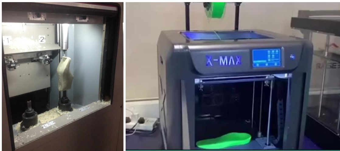
Figure 5: Shoe last processing and 3D printing sole
