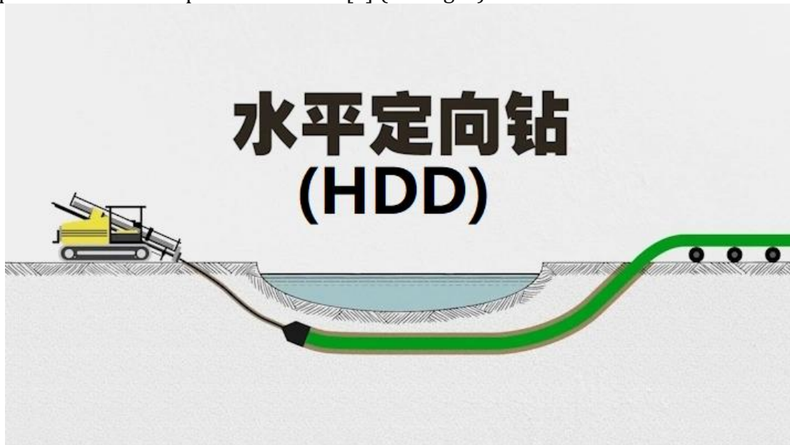
Fig. 1 Schematic diagram of HDD underground pipeline installation method
