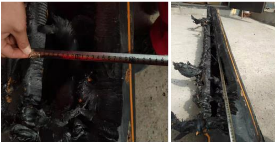
Fig. 3 Damage to pipes caused by existing HDD boreholes
