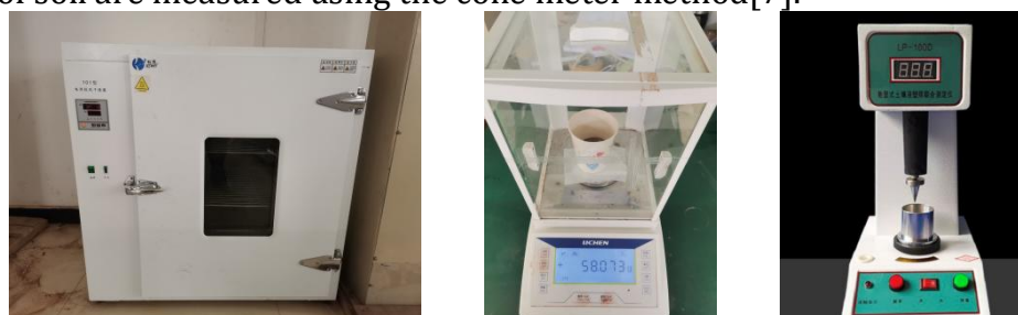
(a)Electric heating blast drying oven (b)Electronic scale (c)Cone meter Figure 4 Relevant experimental equipment
