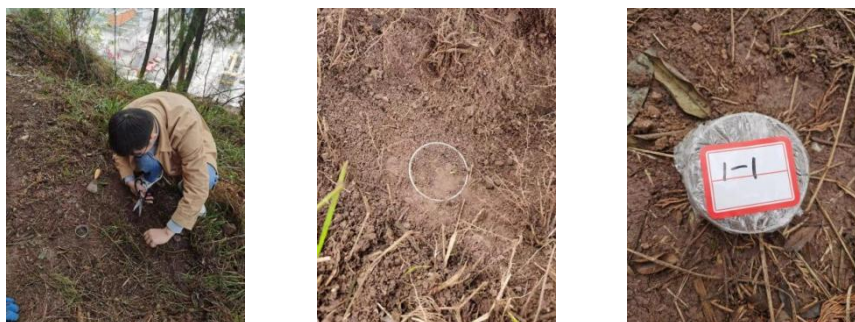
(a)Clean up humus soil (b)Ring knife pressed in (c)Sampling and numbering Figure 3 Sampling process of intact ring knife
