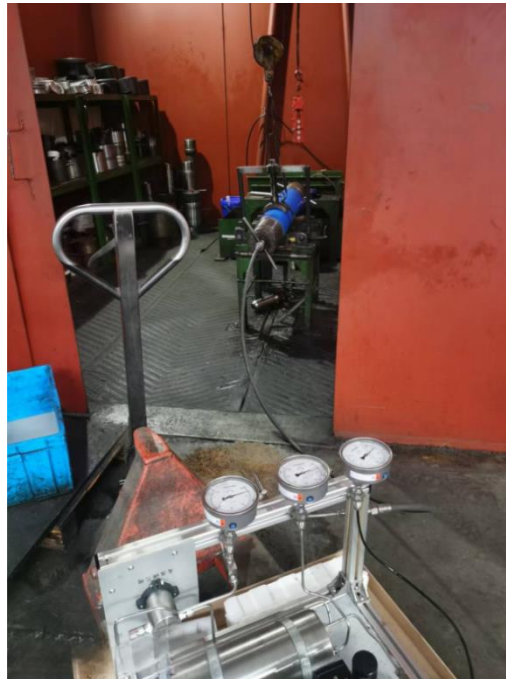
Figure 6 Pneumatic Seal Integrity Test
