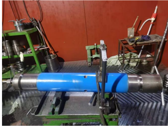
Figure 4 Tool hydraulic Seal Performance Test
