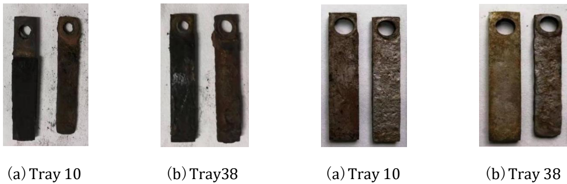
Figure 2 Appearance of Corroded Coupons Figure 3 Appearance of Pickled Coupons
