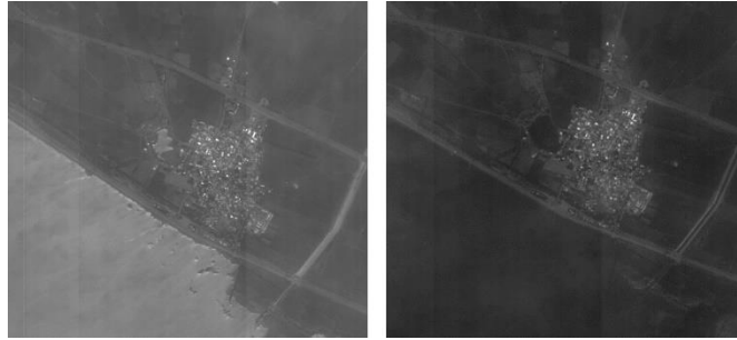
Fig. 13 Radiometric differences of the same ground object across different satellite frames
