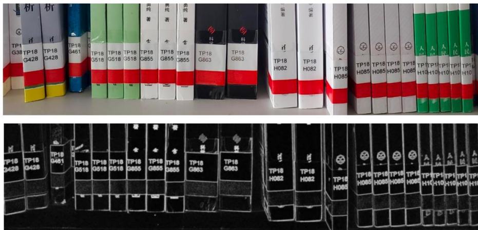
Fig. 4 Input image of book spines and the corresponding edge detection result
