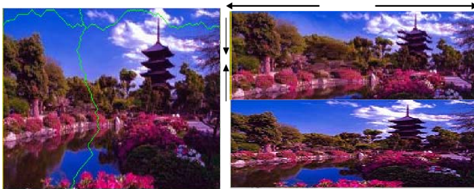
Fig. 2 The image resizing based on seam carving algorithm
