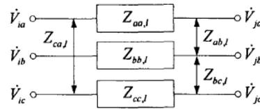
Fig.1 Feeder model
