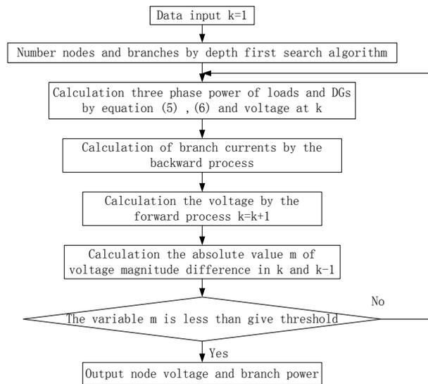
Fig. 3 Flowchart of algorithm
