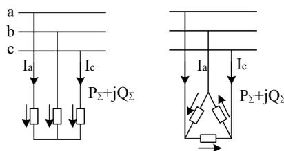
Fig. 2 Load model in ungrounded network
