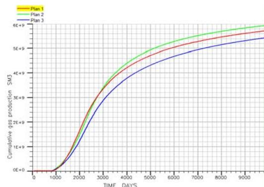
Fig. 3 Cumulative gas production curves of Scheme 1, 2, 3
