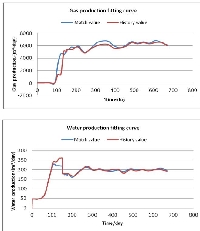
Figure 1. The gas production rate and water rate curve fitting
