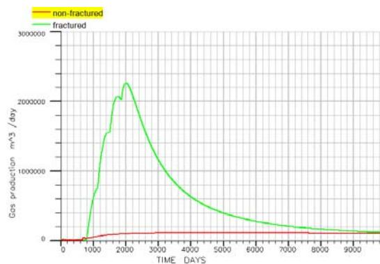
Fig. 2 Gas production curves of fractured and non-fractured
