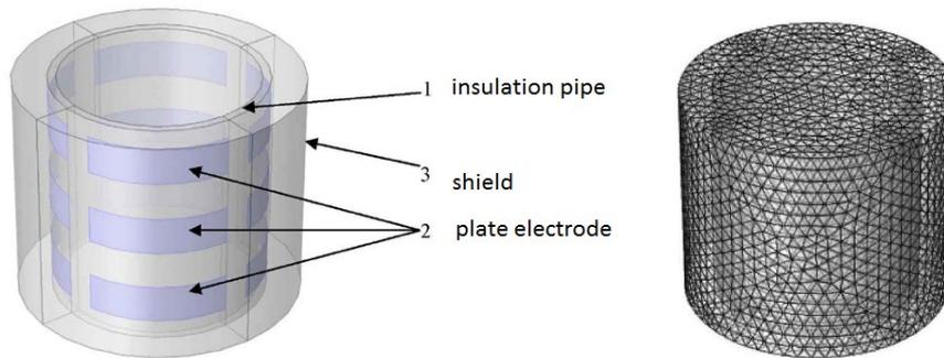
Fig. 1 12 electrodes array for 3D ECT system Fig.2 The finite element mesh
