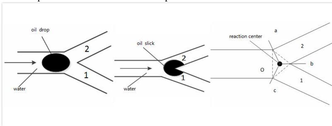
Fig. 2 Two channel selection model of oil droplets or oil film
