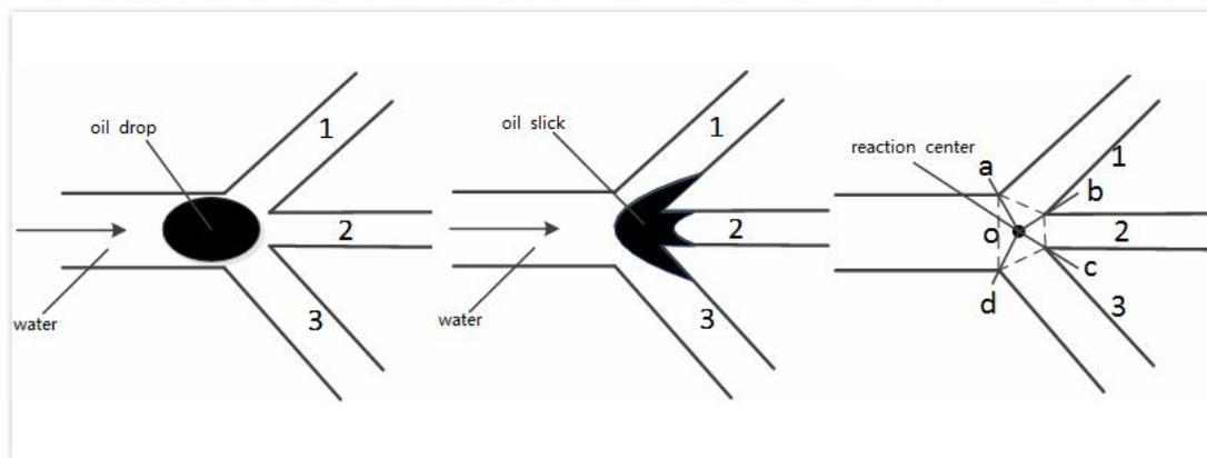
Fig. 3 Two channel selection model of oil droplets or oil film
