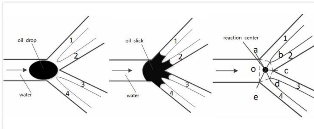
Fig. 4 Two channel selection model of oil droplets or oil film
