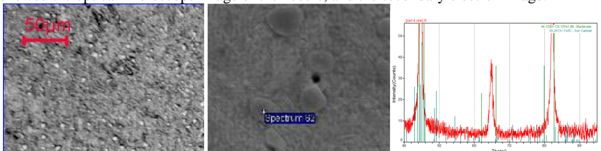
Figure 1. Microstructure analysis of German needles (a) Optical microscope, (b) SE (secondary electron), and (c) the X-ray energy spectrum
