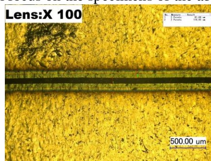
Figure 4: Kerf width focus in - 1 position
