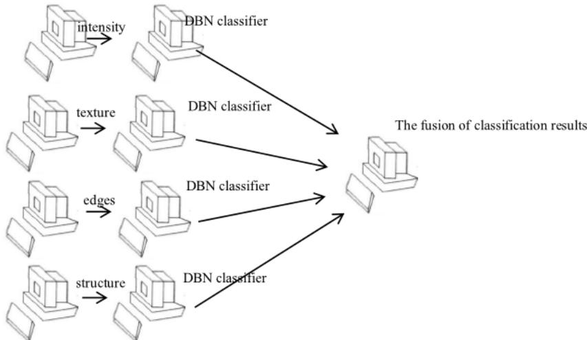
Fig. 2 Structure of target detection system based on MAS
