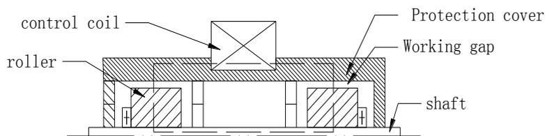
Fig. 2 Circuit structure of the damper
