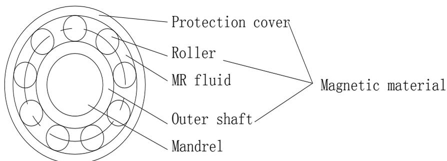
Fig. 3 Structure diagram of working part in MR damper
