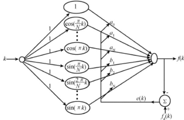
Fig. 1 BP neural network model based on Fourier basis function
