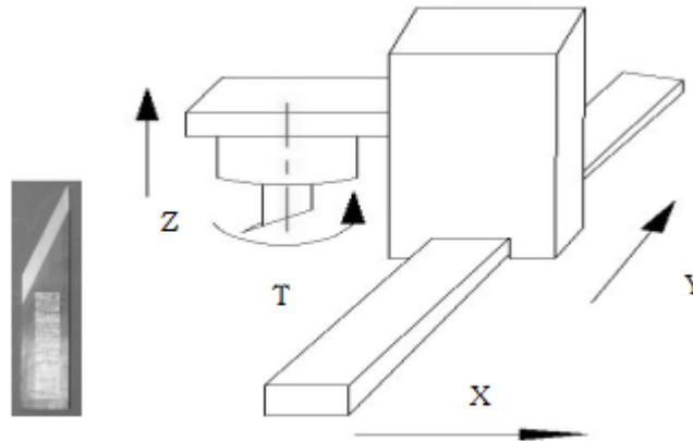
Fig. 1 Cutter and the structural model of proofer
