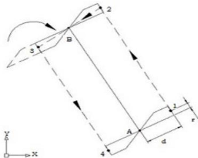
Fig. 2. Trajectory of V cutter
