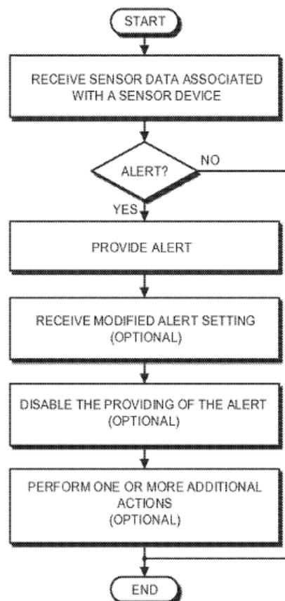
Fig. 3 flow diagram illustrating a method for providing an alert based on an alert setting
