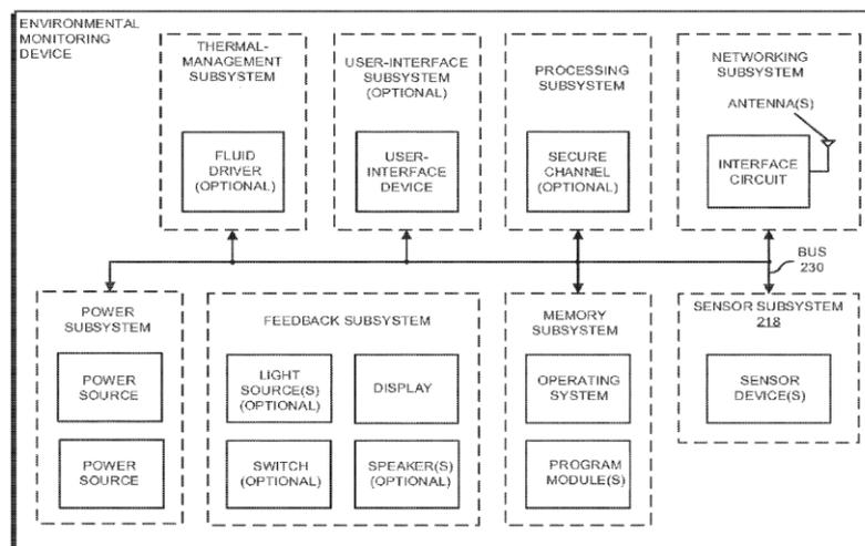
Fig. 1 block diagram illustrating an environmental monitoring device
