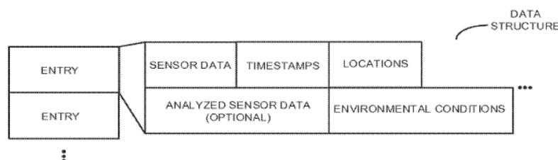
Fig. 2 block diagram illustrating a data structure with sensor data
