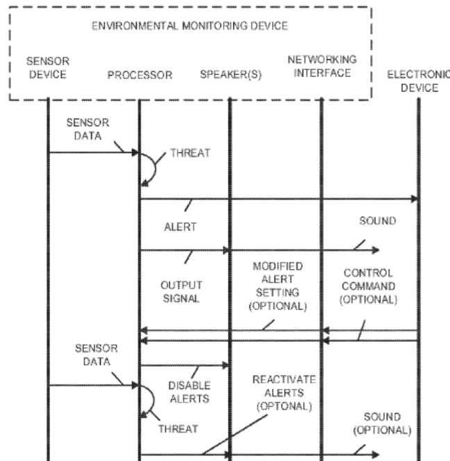
Fig. 4 is a drawing illustrating communication between an environmental monitoring device and an electronic device during the method
