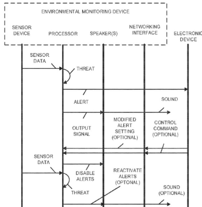
Fig. 4 is a drawing illustrating communication between an environmental monitoring device and an electronic device during the method
