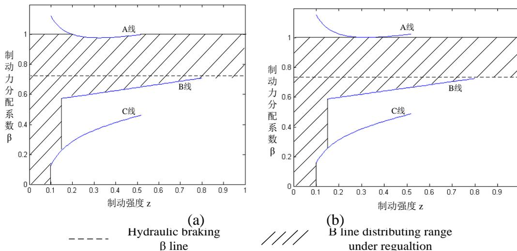
Fig.3 Relationship between braking force distribution coefficient  $\beta$  and braking intensity  $z$
