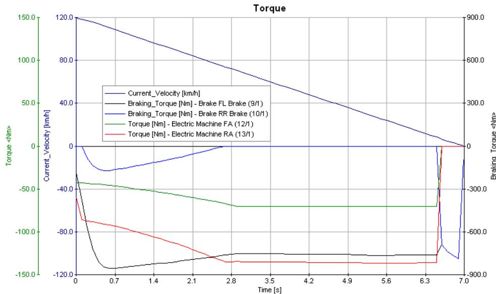
Fig.10 Relationship between vehicle speed and brake torque when the braking intensity is 0.6g
