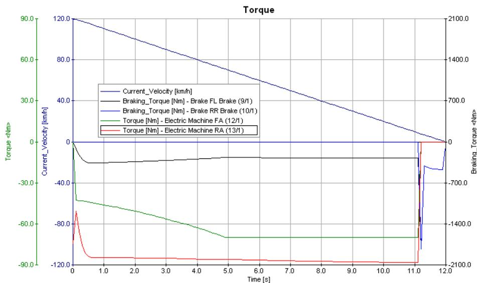
Fig.9 Relationship between vehicle speed and brake torque when the braking intensity is 0.3g
