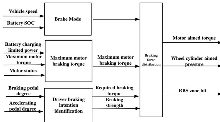
Fig.4 Flow charts of braking energy recovery control algorithm
