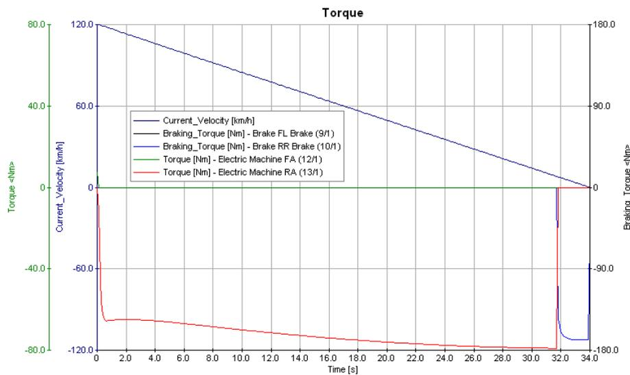
Fig.8 Relationship between vehicle speed and brake torque when the braking intensity is 0.1g
