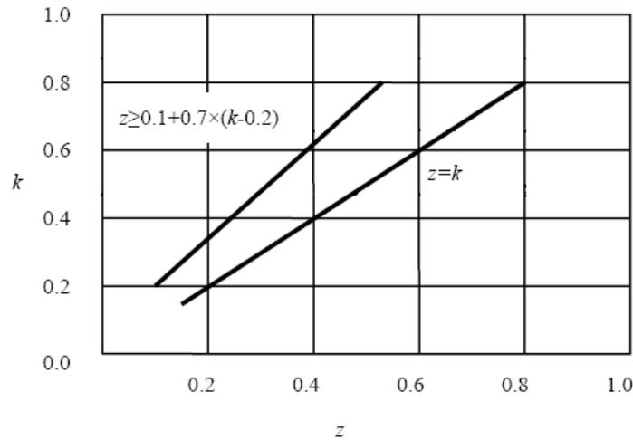
Fig.2 Braking force distribution in ECE Regulations
