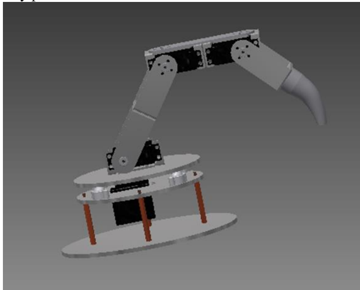
Fig.3 The structure of spray-painting manipulator
