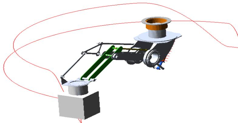
Fig. 3 Robot simulation trajectory
