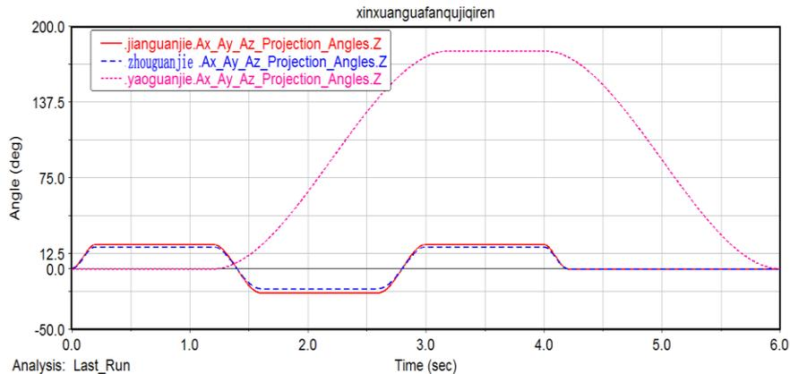
Fig. 7 Angle variation curve of each link
