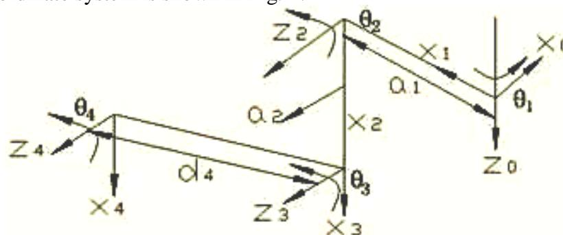
Fig. 4 Robot link coordinate system
