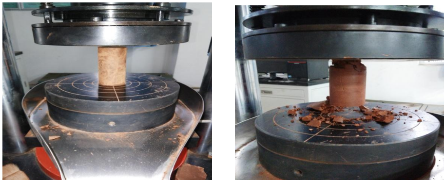
Figure3 cylinder rock uniaxial compressive test
