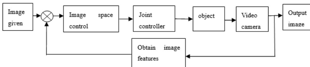
Fig. 2 the servo structure based on image control
