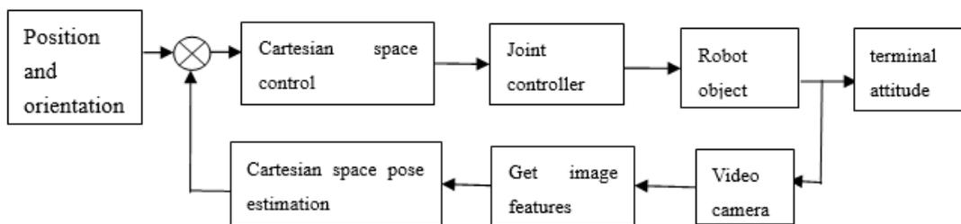
Fig. 1 the structure of the servo system based on the position control
