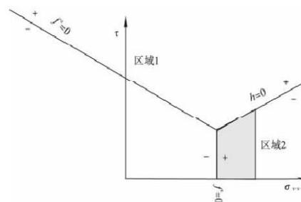
Figure 2 flow rule of Joints weak surface of Ubiquitous - joint model
