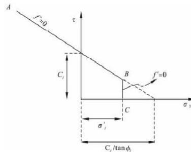
Figure 1 yield criterion of weak joint surface
