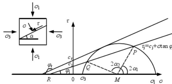
It can be seen, when the joint angle  $\alpha_1 < \alpha < \alpha_2$ , the destruction of jointed rock mass mainly controlled by the joint surface; when the joint angle  $\alpha < \alpha_1$  or  $\alpha > \alpha_2$ , the destruction of jointed rock mass is almost unaffected by joint plane, but controlled by the rock strength.
