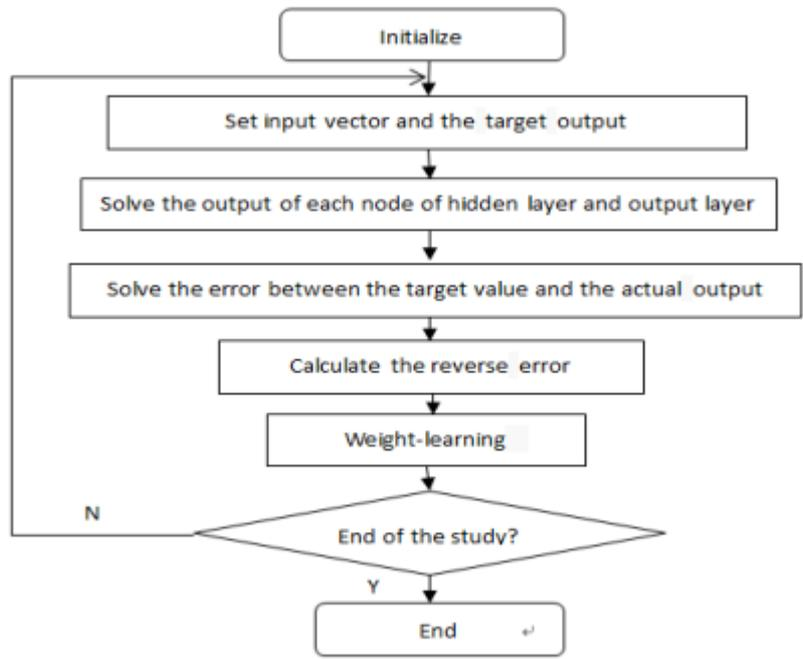
Fig.2 The BP neural network algorithm flow chart
