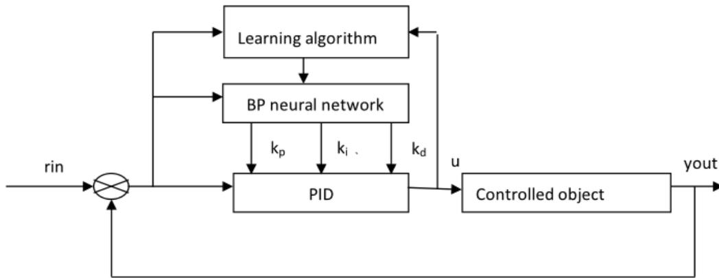
Fig. 3 The structure diagram of the BP neural network PID controller
