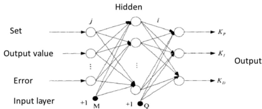
Fig.1 The structure of the BP neural network
