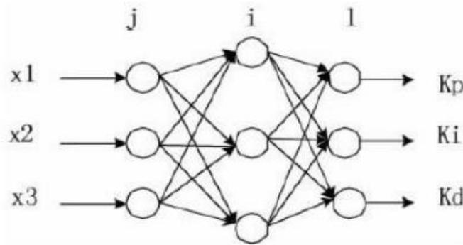
Fig. 4 Three layer BP neural network structure
