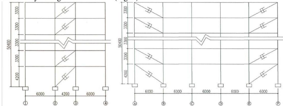
Fig. 2 Viscous damper arrangement scheme
