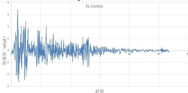
Fig. 3 EL-Centro seismic wave (wave length is 0.02s, and the duration is 54s)
