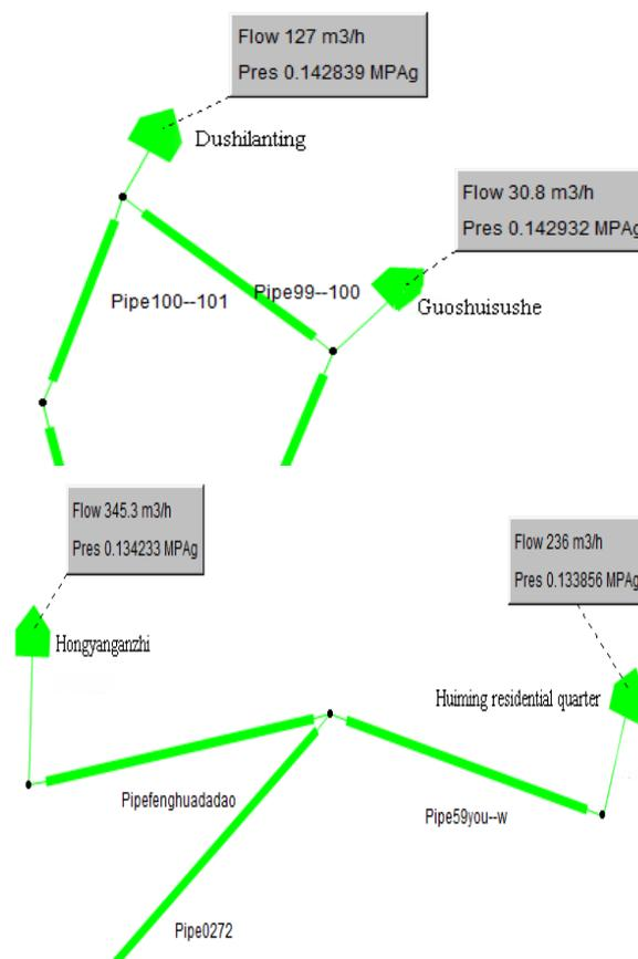
Fig. 1 Pressure distribution of medium-pressure main pipe
