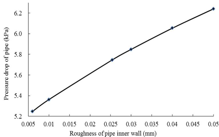
Fig. 2 Rule of the pressure drop with the roughness of pipe inner wall
