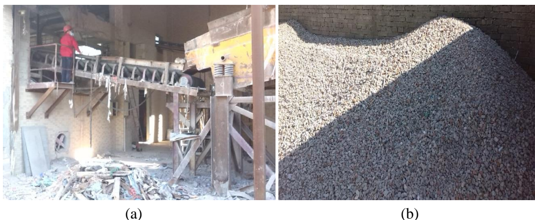
Fig.2 The crushing process of construction waste (a) and the construction waste recycled aggregates (b).
