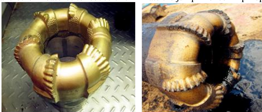
Fig. 7 Eighth run in hole coring bit and pull out coring bit
