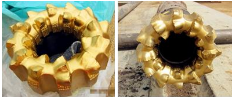
Fig. 2 DFC1312 type PDC coring bits and DFC1312 scalloped type PDC coring bits
