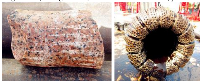
Fig. 6 Seventh taking core and pull out coring bit
