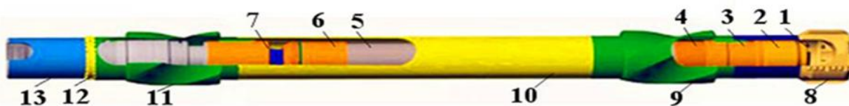
1.Core Catcher 2.3.4. Inner Barrel Shoe Assembly 5. Fiberglass inner tube 6. Inner Tube top sub 7.Rotary Assembly 8.Coring Bit 9. Lower Stabilizer 10.Coring Outerbarral 11. Top Stabilizer 12. Friction Ring 13.Safty Sub
