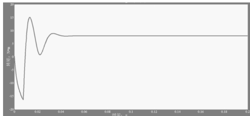
Fig. 4 torque output curve of permanent magnet synchronous motor
