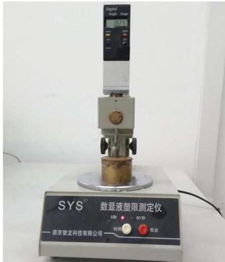
Fig. 2 Liquid-plastic limit determination test of silt
