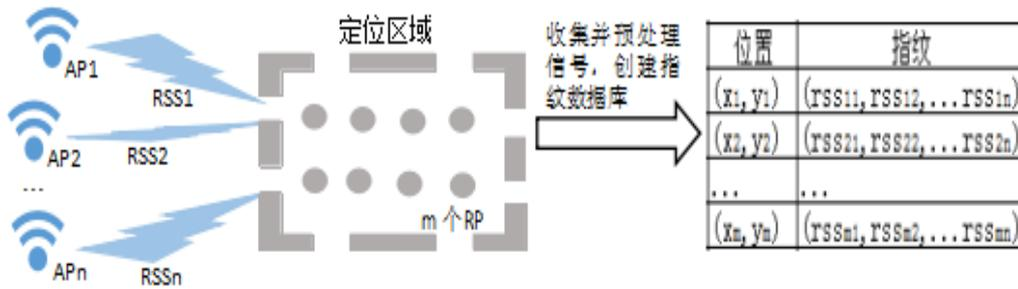
Fig.1 The establishment of the fingerprint database
