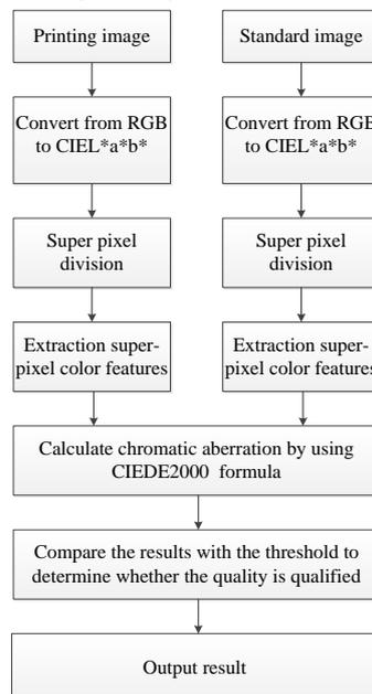
Fig.1 Flow chart of chromatic aberration detection algorithm based on super-pixel
